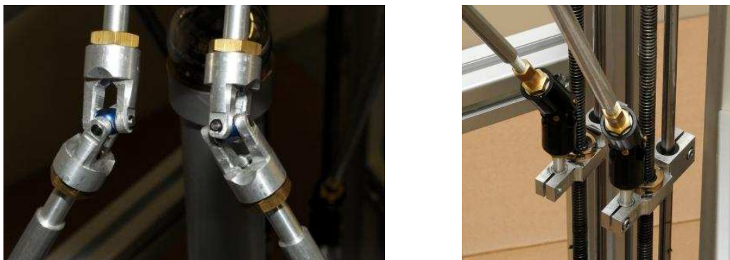
Fig. 4: Cardan joints at the upper (left) and lower ends of abutments (right)
